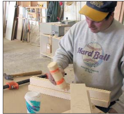
Here an employee glues up panels for doors. Cherry has been the most popular material for kitchen cabinets in recent months, says Joni Van Dusartz.
